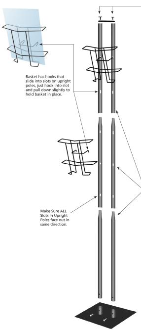
Screw in top support to hold poles in place.
