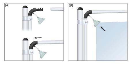
Spring tension holds graphic in place (maximum.020pointgraphicthickness).
